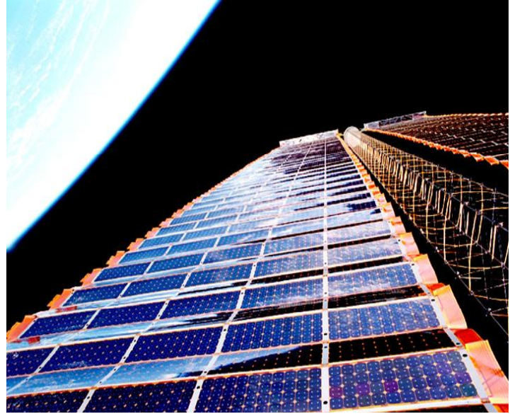
Looking out across an ISS Solar Array Size: 12 m wide x 36.5 m in Length
